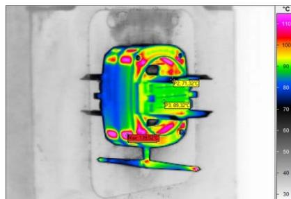
Fig. 5 Thermogram of the moulded part at 80 °C mould temperature and 25 s total cooling time
