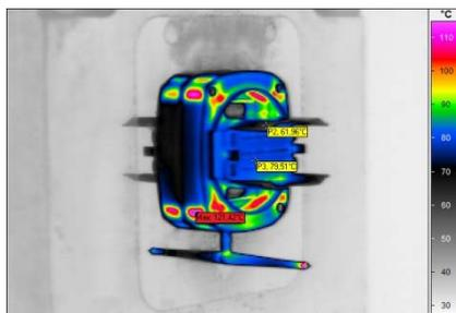
Fig. 4 Temperature-time sequence of the moulded part at 60 °C mould temperature and 25 s total cooling time
